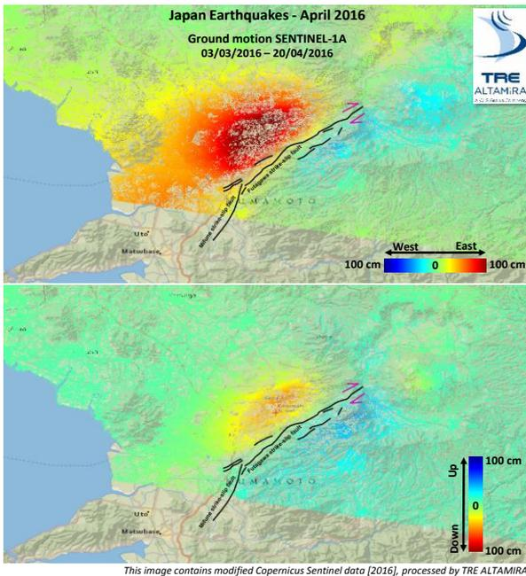
Figure 8. West-East and Up-Down motion maps of Japan's earthquake, using ascending and descending orbits.
