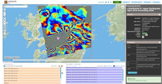
Figure 5. DIAPASON ascending interferogram of Japan earthquakes.
