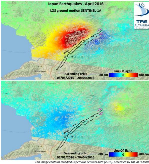
Figure 7. Ascending and Descending LOS motion maps of Japan's earthquake.
